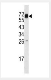
Western blot analysis of CD105 antibody (Center E395) in mouse heart tissue lysates (35  $\mu$ g/lane). CD105 (arrow) was detected using the purified pAb.
