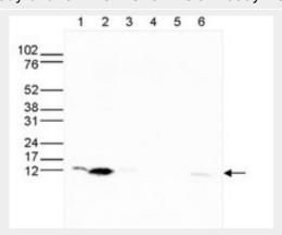
Western blot was performed on whole cell (25  $\mu$ g, lane 1) and histone extracts (15  $\mu$ g, lane 2) from HeLa cells, and on 1  $\mu$ g of recombinant histone H2A, H2B, H3 and H4 (lane 3, 4, 5 and 6, respectively) using the antibody The marker (in kDa) is shown on the left.
