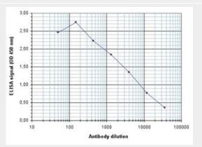
To determine the titer, an ELISA was performed using a serial dilution of the antibody. The antigen used was a peptide containing the histone modification of interest. By plotting the absorbance against the antibody dilution the titer of the antibody was estimated to be 1:4,000.
