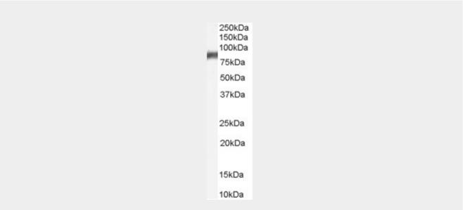
AF1092a (0.3  $\mu$ g/ml) staining of Rat Stomach lysate (35  $\mu$ g protein in RIPA buffer). Primary incubation was 1 hour. Detected by chemiluminescence.
