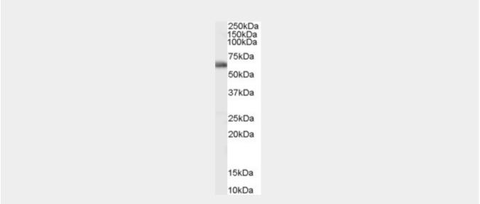
AF1699a (0.1  $\mu$ g/ml) staining of Human Bone Marrow lysate (35  $\mu$ g protein in RIPA buffer). Primary incubation was 1 hour. Detected by chemiluminescence.
