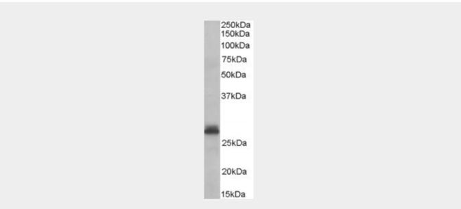
AF2062a (0.3  $\mu$ g/ml) staining of Human Heart lysate (35  $\mu$ g protein in RIPA buffer). Primary incubation was 1 hour. Detected by chemiluminescence.
