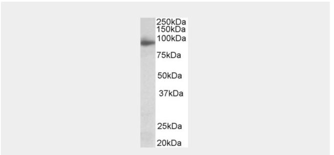
AF3794a (1  $\mu$ g/ml) staining of Amygdala lysate (35  $\mu$ g protein in RIPA buffer). Primary incubation was 1 hour. Detected by chemiluminescence.
