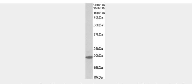
AF3876a (0.3  $\mu$ g/ml) staining of MOLT4 lysate (35  $\mu$ g protein in RIPA buffer). Primary incubation was 1 hour. Detected by chemiluminescence.
