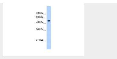
WB Suggested Anti-IFIT3 Antibody Titration: 0.25µg/ml
