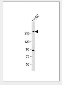
Anti- at 1:1000 dilution + HepG2 whole cell lysate Lysates/proteins at 20  $\mu$ g per lane. Secondary Goat Anti-mouse IgG, (H+L), Peroxidase conjugated at 1/10000 dilution. Predicted band size : 273 kDa Blocking/Dilution buffer: 5% NFDM/TBST.
