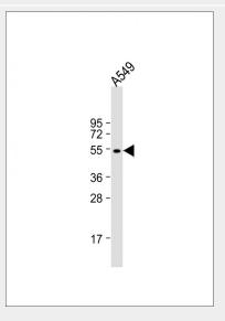
Anti-ACVR1 Antibody (Center) at 1:2000 dilution + A549 whole cell lysate Lysates/proteins at 20  $\mu$ g per lane. Secondary Goat Anti-Rabbit IgG, (H+L), Peroxidase conjugated at 1/10000 dilution. Predicted band size : 57 kDa Blocking/Dilution buffer: 5% NFDM/TBST.
