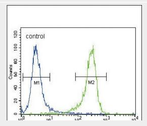
UCHL1 Antibody (N-term) (Cat. #AP2126a) flow cytometric analysis of NCI-H460 cells (right histogram) compared to a negative control cell (left histogram).FITC-conjugated goat-anti-rabbit secondary antibodies were used for the analysis.
