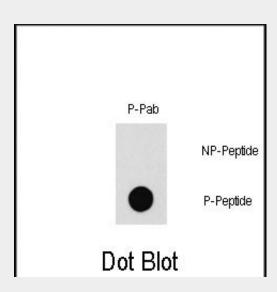
Dot blot analysis of Phospho-PAK1-T212 Pab (Cat.AP3328a) on nitrocellulose membrane. 50ng of Phospho-peptide or Non Phospho-peptide per dot were adsorbed. Antibody working concentrations are 0.5ug per ml.
