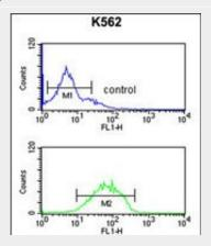
HHAT Antibody (N-term) (Cat. #AP5503a) flow cytometric analysis of K562 cells (bottom histogram) compared to a negative control cell (top histogram).FITC-conjugated goat-anti-rabbit secondary antibodies were used for the analysis.
